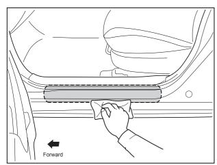
Open the front door and clean the ① scuff plate mounting surface using a cloth soaked in white gasoline or neutral detergent. Then dry it completely.
